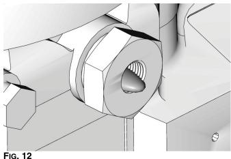
3. Tighten pump element fitting using two wrenches working in opposite directions (FIG. 11).
